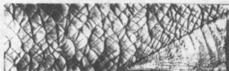
Fig. 2. Cellular pattern with \theta = 19.3^\circ wedge
