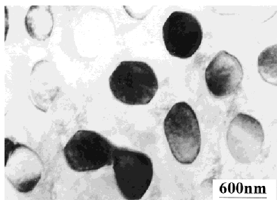
FIG. 3. Bright-field TEM micrograph showing morphology of TiC particles in the eutectic austenite at a 15-mm/s beam scanning speed.
