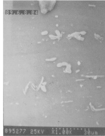
Fig.1 Microcracks on a section of an impacted aluminium alloy specimen
