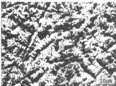
Fig.4 Segregation of TiCp particles in dendritic zone at 4 mm/s beam scanning speed
