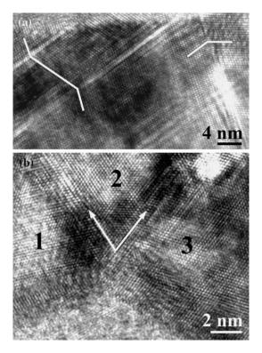
**Fig. 3** HRTEM images showing (a) two twinning systems and (b) threefold twin. The twin boundary is indicated by arrows and each twin domain is numbered (1–3)
