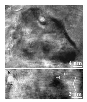
Fig. 2 (a) HRTEM image showing a nc grain with its lower part transforming into a twin. The arrow indicates the twin boundary. (b) Enlarged view showing the details of the twin. Note the presence of a dislocation dipole near the twin boundary
