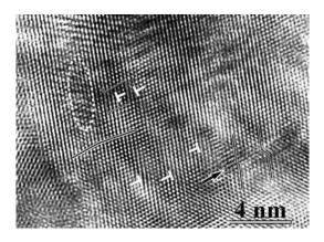
Fig. 4 HRTEM images showing the co-existence of full dislocations and a microtwin indicated by an arrow. Also note the presence of local severe lattice distortion (circled)
