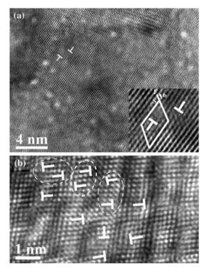
Fig. 1 (a) HRTEM micrograph showing the presence of one dislocation dipole in a nc Ni grain after LNT tensile test. The dislocations are indicated by "Ts". Inset is an enlarged view of dislocation with a Burgers circuit, starting from S and finishing at F, around the dislocation core. (b) HRTEM micrograph showing dislocations on (111) plane of a nc grain of grain size 30 nm. Note that most dislocations form dipoles (some are circled)
