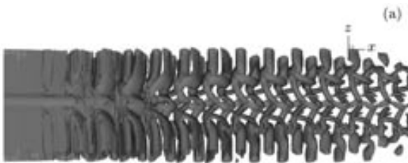
Fig. 1. Iso-surface of |\omega| = 0.12 in the full calculation region at t = 300 .
