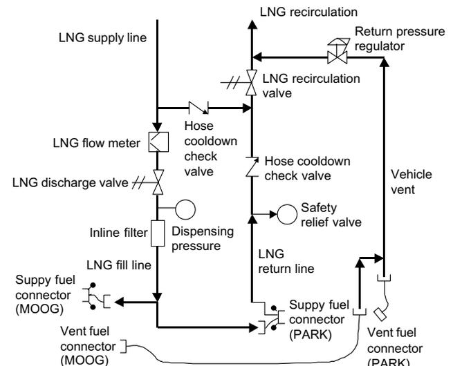
Fig. 1. LNG dispenser module with MOOG and PARK fuel connectors.
