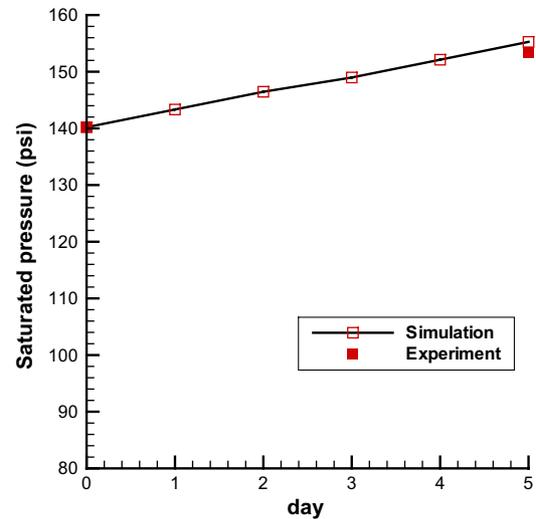
Fig. 5. Predicted saturated pressure for a 15,000 gal tank with an initial fill of 2571 gal LNG at saturated pressure of 140.2 psi and  $C = 1$  W/K. Solid symbols are experimental data taken from an LNG station in Beijing.
