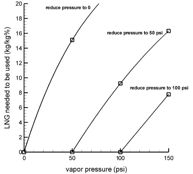
Fig. 4. Percentage of LNG to be boiled to reduce saturated vapor pressure.
