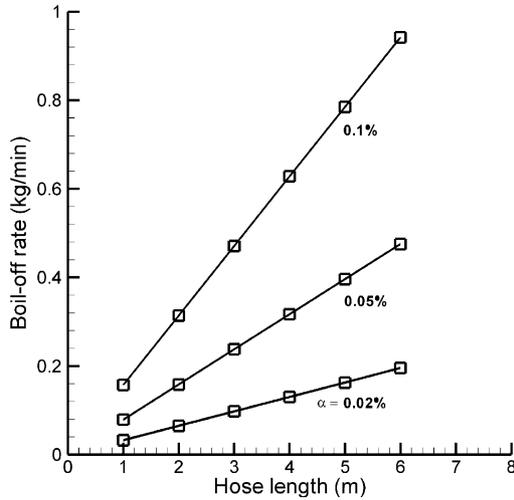
Fig. 3. Boil-off LNG as a function of length of hose to fuel a vehicle.
