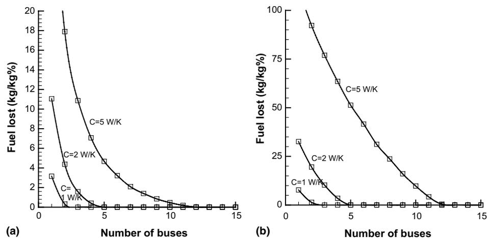
Fig. 6. (a) Total fuel loss and (b) fuel loss per day with number of buses.
