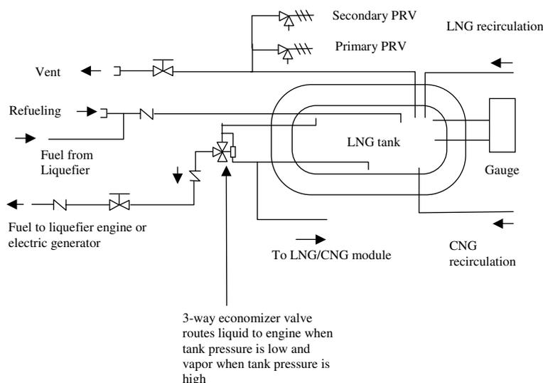
Fig. 7. LNG storage tank with module of electric generator or liquefier.
