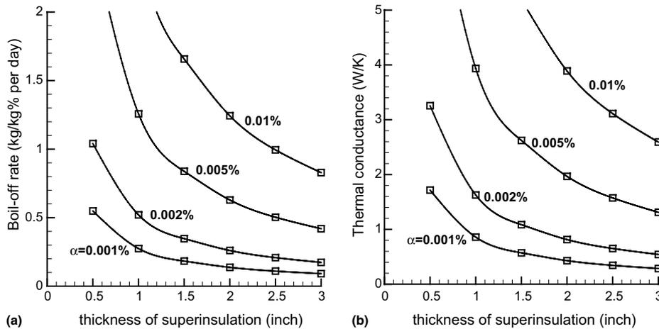
Fig. 2. (a) Boil-off rate and (b) thermal conductance as a function of thickness of multilayer superinsulation for a tank with an area density of  $\beta = 2$ , which is filled with LNG at  $-162$  °C.
