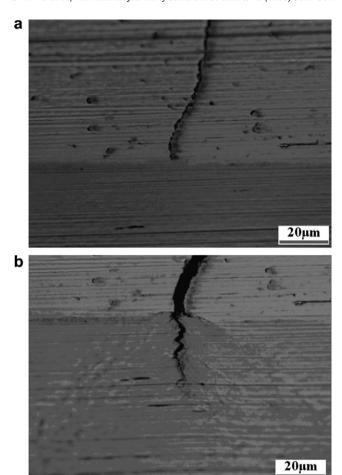
Fig. 8. (a) Coating/interface in initial state. (b) Coating/interface after r4.
