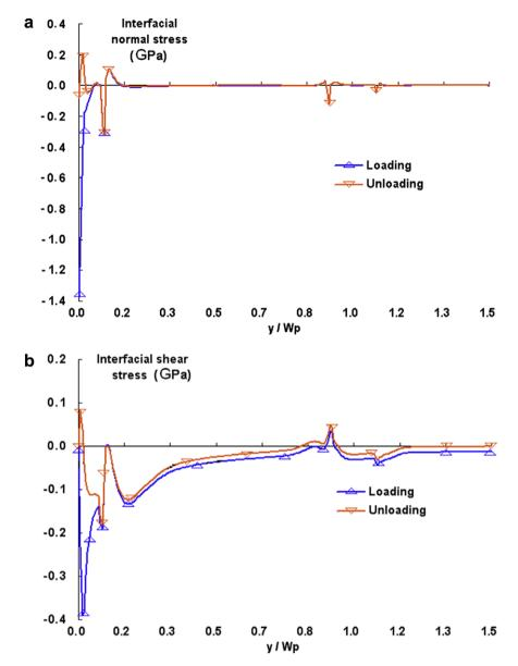
Fig. 12. (a) Interfacial normal for direct bending. (b) Interfacial shear stress for direct bending.
