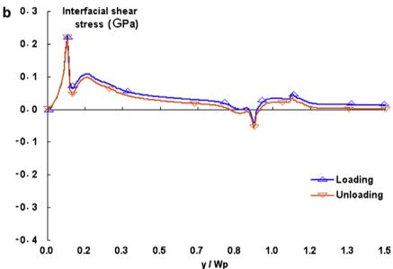
Fig. 13. (a) Interfacial normal stress for reverse bending. (b) Interfacial shear stress for reverse bending.
