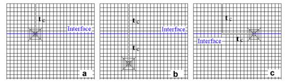
Fig. 14. Sketch of the crack (a) in coating (b) penetrating into substrate (c) deflecting into interface.
