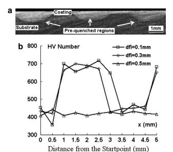
Fig. 1. (a) The profile of the specimen (Fu et al., 2000) and (b) HV number of the surface layer of the substrate as-quenched by CO<sub>2</sub> laser.
