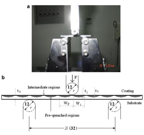
Fig. 2. (a) The loading equipment. (b) Sketch of the specimen.
