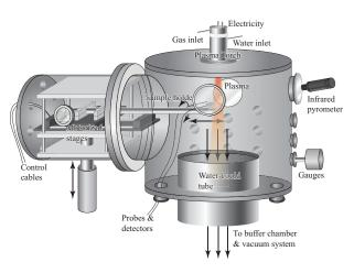
Fig. 1 Schematic of the main part of the 150 kW arc-heated plasma testing facility.
