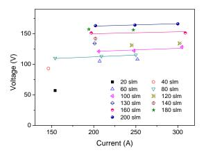
Fig. 3 I-V curves of the  $N_2$  plasma with different gas flow rates.
