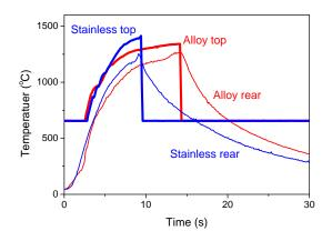
Fig. 6 Time dependent top and rear surface temperature of the TPM samples in the test. The samples were moved out of the plasma jet after the test, and the top surface temperature was no longer monitored by the pyrometer.
