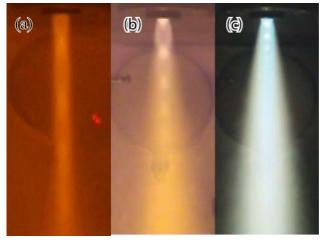
Fig. 2 Photos of plasma jets under different chamber pressures and gas compositions. (a)  $N_2$ , 1 kPa; (b)  $N_2$ , 10 kPa; (c) 20 %vol  $O_2$ - $N_2$ , 30 kPa.
