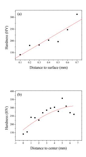
Fig. 8 Micro Vickers hardness distributions of Ni-base alloy samples after test. (a) along the thickness direction; (b) along the surface direction.
