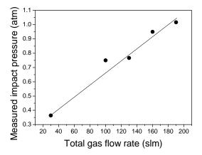
Fig. 5 Dependence of the measured impact pressure on the total gas flow rate.
