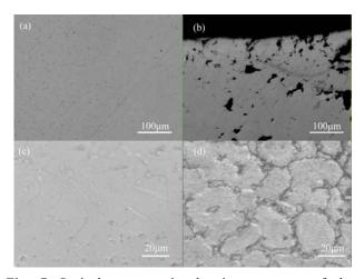
Fig. 7 Optical cross-sectional microstructures of the Ni-base refractory alloy before and after stagnation ablation test. (a) before ablation, not etched (b) after ablation, not etched (c) before ablation, etched (d) after ablation, etched.
