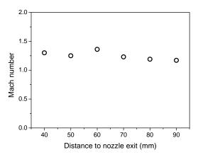
Fig. 4 Axial Mach number distributions in N2 plasma jet at 1 kPa.
