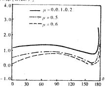
Fig. 2 The angular distribution of mean Fig. 3 The angular distribution of effective stress for various values of  $\mu$
