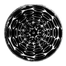
(c1) Theoretical contour of (7, 6) mode (f=18.741Hz). (c2) Experimental contour of (7, 6) mode (f=52Hz). Fig.6. Comparison of theoretical contours of surface wave mode with those in experiment (depth of fluid h=1.0 cm, radius of the vessel R=7.5 cm, the forcing amplitude  $A=11.4\mu$ m).
