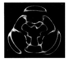
(a<sub>1</sub>) Theoretical contour of (3, 3) mode (f=11.68Hz). (a<sub>2</sub>) Experimental contour of (3, 3) mode (f=20Hz).
