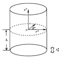
Fig.1. Physical model of the liquid-filled circular cylinder.
