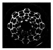
(b<sub>2</sub>) Experimental contour of (8, 4) mode (f=50Hz).
