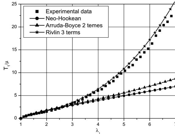
Fig. 11. Comparison between experimental data and models for uniaxial tension.
