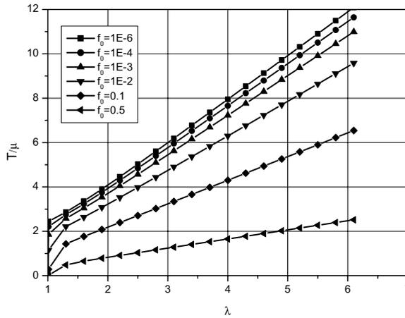
Fig. 5. Neo-Hookean laws for hydrostatic tension with different fixed initial porosities  $f_0$ .
