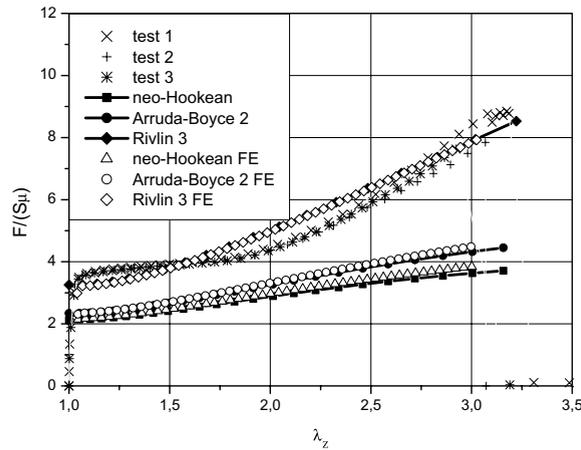
Fig. 13. Comparison between experimental data and models for pancake tests.
