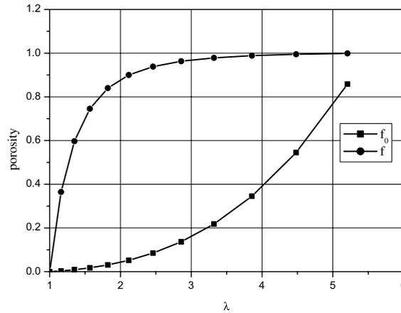
Fig. 7. Variation of  $f_0$  and  $f$  for hydrostatic tension,  $n = 20$ .
