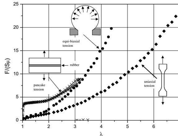
Fig. 10. Experimental results for uniaxial, equi-biaxial and pancake tests.  $F/(S\mu)$  denotes the normalized nominal engineering stress.
