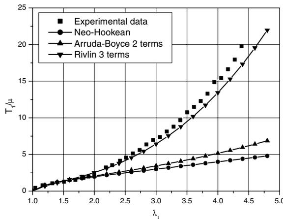
Fig. 12. Comparison between experimental data and models for equi-biaxial tension.
