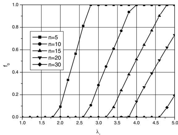
Fig. 4. Evolution of the porosity  $f_0$  for different  $n$  under equi-biaxial tension.
