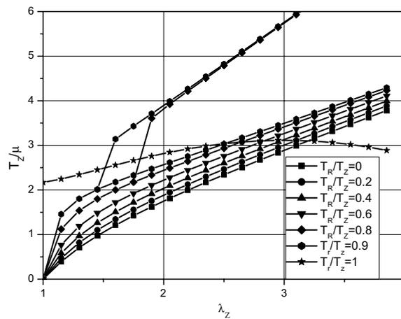
Fig. 9. Neo-Hookean laws for stress-imposed cylindrical tensions.
