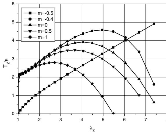
Fig. 8. Neo-Hookean laws for strain-imposed cylindrical tensions.
