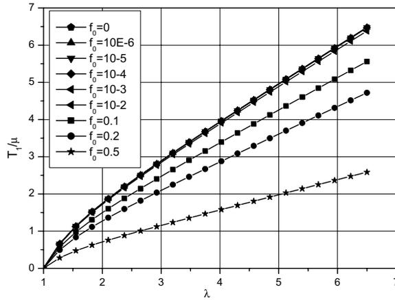
Fig. 1. Neo-Hookean laws for uniaxial tension with different fixed porosities  $f_0$ .
