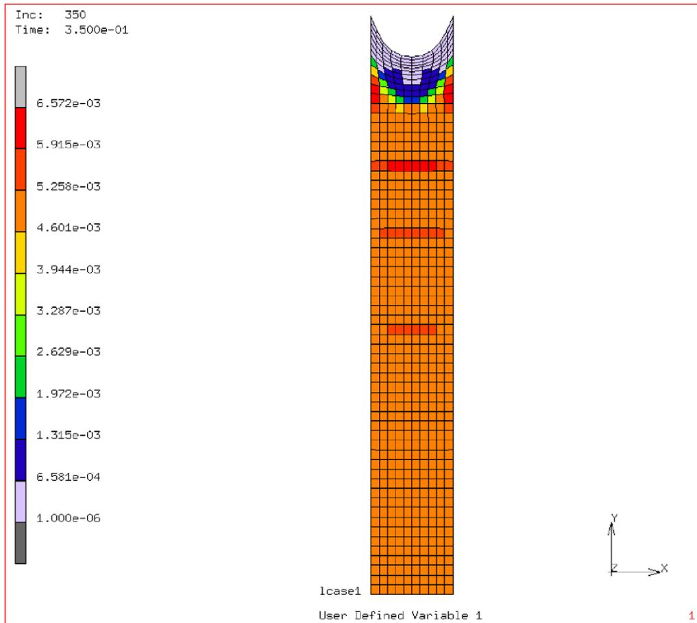
Fig. 14. Porosity distribution and deformation of the pancake specimen.
