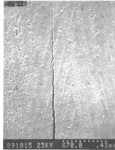
Figure 1 Mode I interlaminar crack propagation in T300/MBMI [0] 26 specimen. The crack propagation direction is upwards
