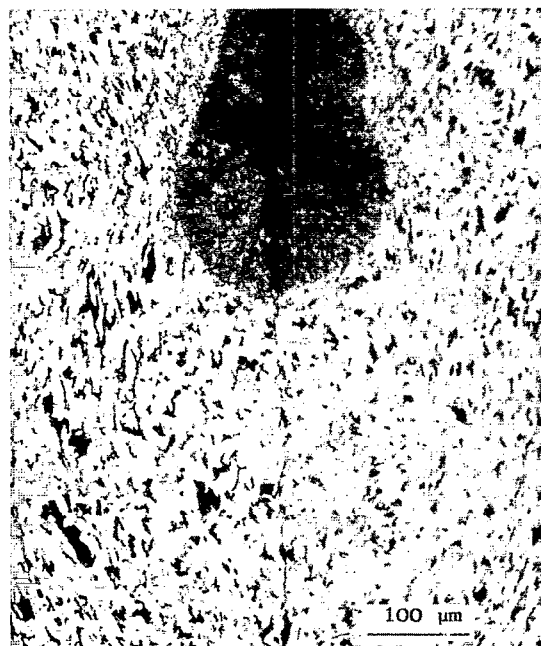
FIG. 9. The morphology of the section perpendicular to the axis of the compact that was consolidated with pickled wires. The upper dark area is the high-temperature area, a white layer around the dark area is pure ferrite. Below it is nonmelting welding.
