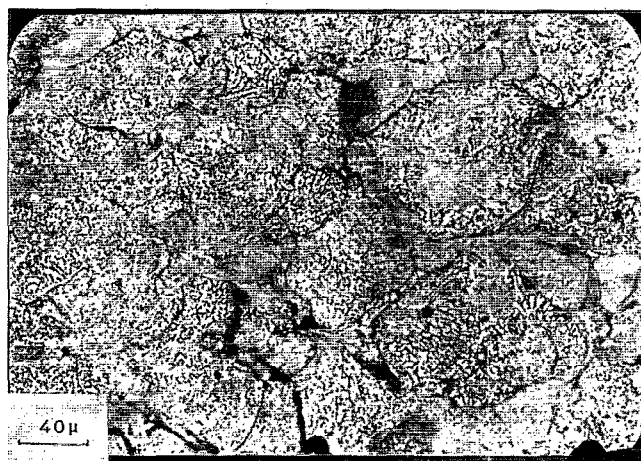
FIG. 15. Microphotograph of explosive compact of 316L stainless steel powder.
