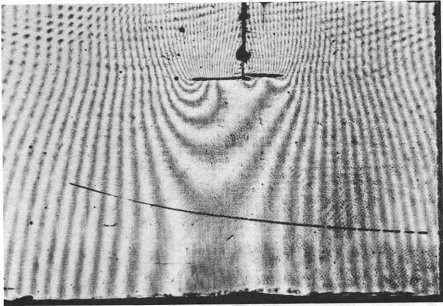
Fig. 7. U and V displacement fields for 0°-ply S1:N carbon/epoxy specimen with longitudinal crack at notch tip.
