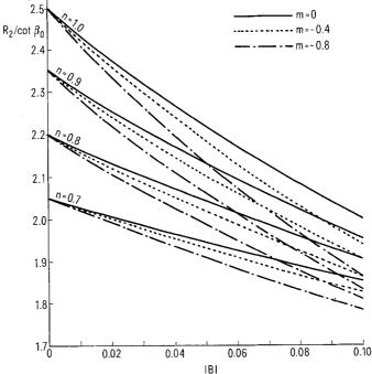
Figure 1 The critical Reynolds number  $R_2/\cot \beta_0$  as a function of elastic parameter |B| for various values of n and  $m (\leq 0)$
