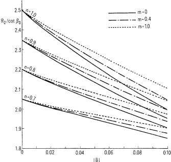
Figure 2 The critical Reynolds number  $R_2/\cot \beta_0$  as a function of elastic parameter |B| for various values of n and  $m \ (\ge 0)$
