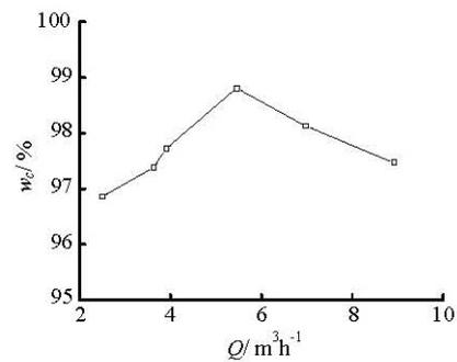
Fig.7 Effect of input flow rate on watercut in the underflow
