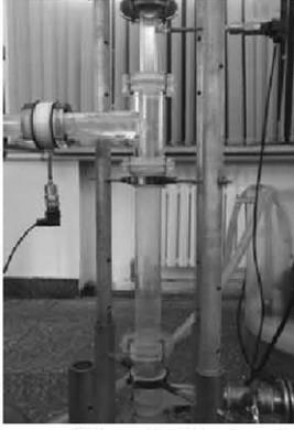
Fig.3 Picture of the cylindrical cyclone in lab
