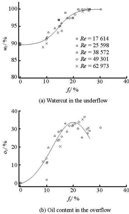
Fig.11 Relationships between flow split-ratio and oil/water separation
