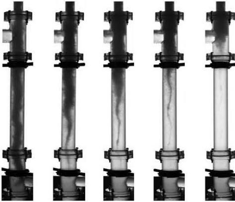
Fig.4 Oil core in the cyclone versus flow split-ratio (from 15.7% to 35.6%)
