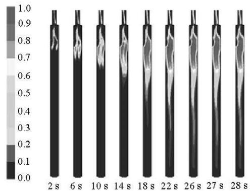
Fig.8 Transient development of oil core structure from numerical simulations
