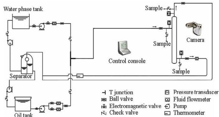
Fig.2 Schematic diagram of the test facility
