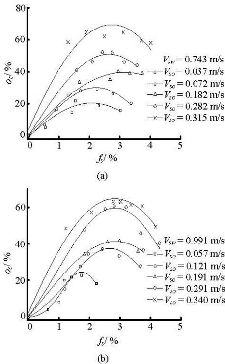
Fig.6 Oil content ( $o_c$ ) in the overflow versus flow split-ratio
