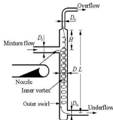
Fig.1 Schematic plot of the cylindrical cyclone
