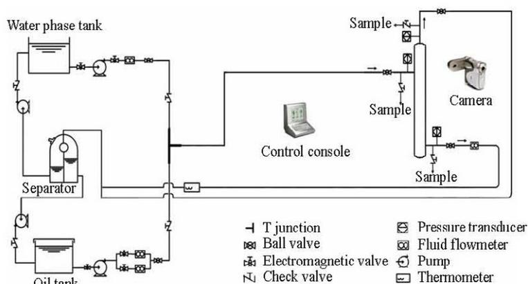
Fig.2 Schematic diagram of the test facility
