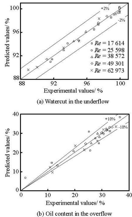
Fig.12 Comparison of experimental and predicted values of oil/water separation in cylindrical cyclone
