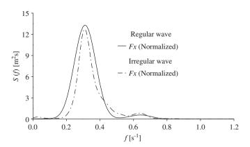
**Fig. 15.** Comparison of amplitude spectra between regular and irregular waves (H/d=0.06).
