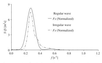
Fig. 18. Comparison of amplitude spectra between regular and irregular waves.
