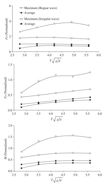
**Fig. 16.** Average and maximum normalized horizontal force (top), vertical force (middle) and moment (bottom).
