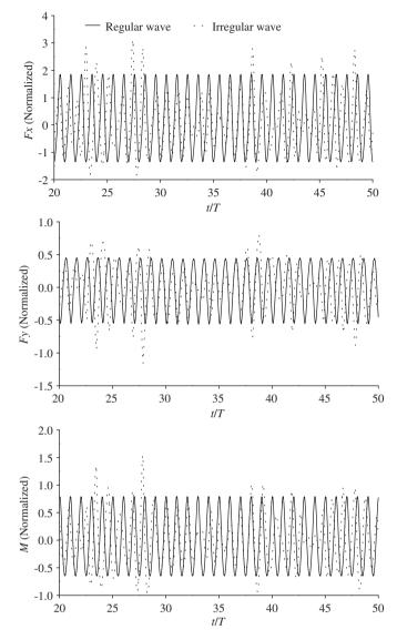
Fig. 12. Time series of calculated normalized horizontal force (top), vertical force (middle) and moment (bottom).
