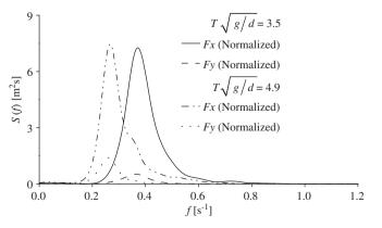
Fig. 17. Amplitude spectra of normalized forces for irregular wave.
