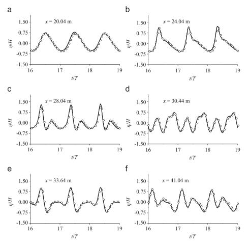
Fig. 6. Comparison of computed and measured free surface elevations over a submerged structure. Numerical solution (solid line), experimental data (circles).
