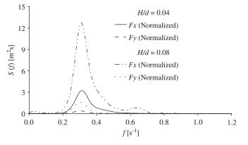
Fig. 14. Amplitude spectra of normalized forces for irregular wave.
