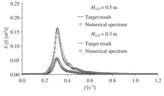
Fig. 4. Comparison of wave spectra.
