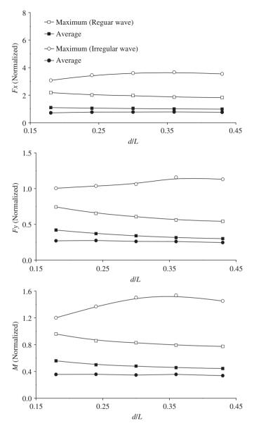
**Fig. 11.** Average and maximum normalized horizontal force (top), vertical force (middle) and moment (bottom) on the structure.
