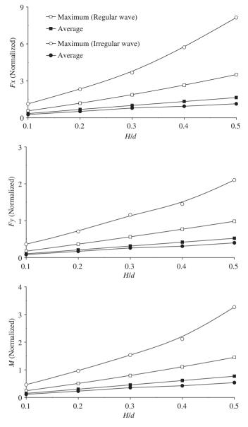
**Fig. 13.** Average and maximum normalized horizontal force (top), vertical force (middle) and moment (bottom) on the structure.
