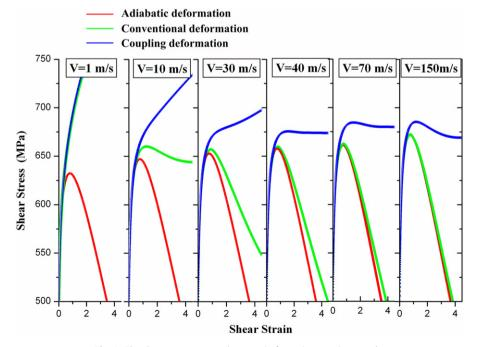
Fig. 6. The shear stress versus shear strain for various cutting speeds.
