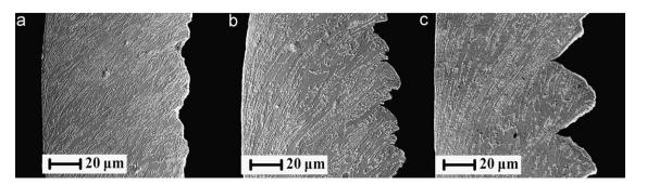
Fig. 3. The SEM microstructure of chip formation at cutting speed of: (a) 30.8 m/s, (b) 38.6 m/s, (c) 67.3 m/s.
