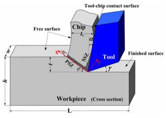
Fig. 2. The schematic diagram of the cutting process.
