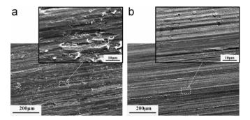
Fig. 5. SEM microstructures of the finished surfaces at cutting speed of (a) 30.8 m/s and (b) 67.3 m/s.
