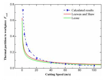
**Fig. 8.** The variation of the heat partition conducted into workmaterial with cutting speed. The heat partition conducted into workmaterial was given as  $F_{work} = 1/(1.13(t/t_c)\sqrt{\rho cVt/2K \sin \varphi})$  by Leone [43] and  $F_{work} = 1-1/(1+1.328\sqrt{K/\rho cVt_c})$  by Loewen and Shaw [44], where  $t_c$  is the chip thickness.
