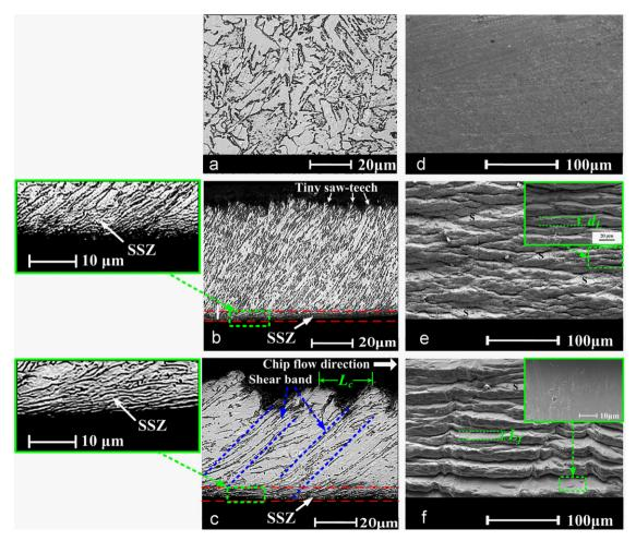
**Fig. 4.** Microstructure of (a) the as-received material, (b, c) the chip obtained at a cutting speed of 30.8 m/s and 67.3 m/s respectively; (d) the free surface of the uncut workpiece; (e, f) the free surface of chips obtained at cutting speed of 30.8 m/s and 67.3 m/s respectively (The free surface is schematically illustrated in Fig. 2.).
