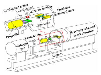
Fig. 1. The experimental system based on the light-gas-loading system.
