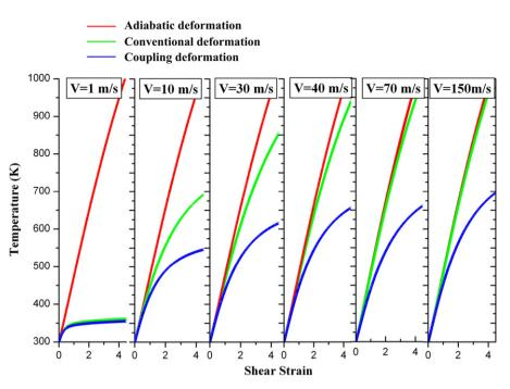
Fig. 7. The temperature versus shear strain for various cutting speeds.
