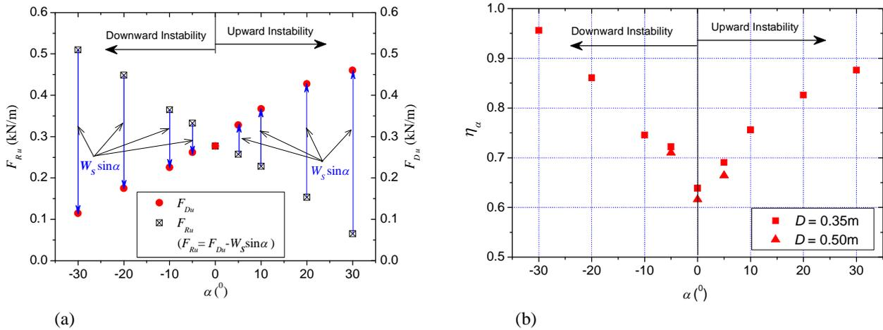
**Fig. 5** Effects of slope angle on the on-bottom stability of anti-rolling pipes: (a) ultimate lateral soil resistance vs. slope angle; (b) lateral-soil-resistance coefficient vs. slope angle ( $D = 0.35$  m,  $W_s = 0.801$  kN/m,  $G = 0.711$  [note:  $W_s = 1.523$  kN/m,  $G = 0.662$ , for  $D = 0.50$  m, see Fig5. (b)],  $\mu = 0.32$ ,  $d_{50} = 0.12$  mm,  $D_r = 0.16$ )
