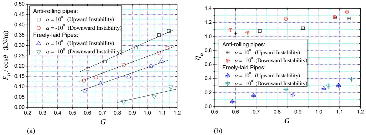
**Fig. 6** Effects of non-dimensional submerged weight and end-constraints of the pipeline on the pipe on-bottom stability: (a) ultimate inclined mechanical load vs. non-dimensional submerged weight of the pipe; (b) ultimate lateral-soil-resistance coefficient vs. non-dimensional submerged weight of the pipe ( $D=0.20$  m,  $\mu = 0.32$ ,  $d_{50} = 0.12$  mm,  $D_r = 0.16$ ).
