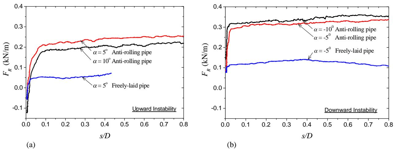
**Fig. 2** The development of lateral soil resistance with increasing lateral displacement while the pipe losing stability on a sloping sand-bed: (a) Upward Instability; (b) Downward Instability. ( $D = 0.35$  m,  $W_s = 0.801$  kN/m,  $G = 0.711$ ,  $\mu = 0.32$ ,  $d_{50} = 0.12$  mm,  $D_r = 0.16$ ).
