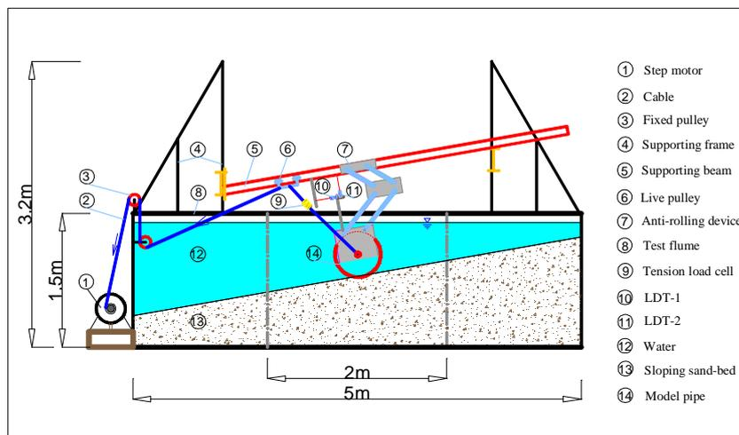
**Fig.1** Schematic diagram of the displacement-controlled experimental setup for pipeline stability on a sloping sand-bed.
