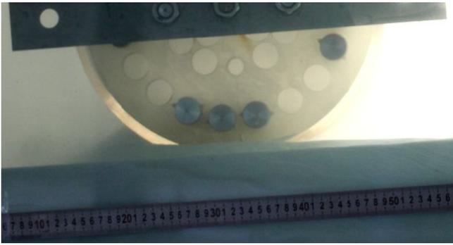
**Fig. 4** Experimental observation of the pipe-soil interaction during pipe losing stability on a sloping sand-bed ( $\alpha = -5^\circ$ ,  $D = 0.35$  m,  $W_s = 0.801$  kN/m,  $G = 0.711$ ,  $\mu = 0.32$ ,  $d_{50} = 0.12$  mm,  $D_r = 0.16$ ).
