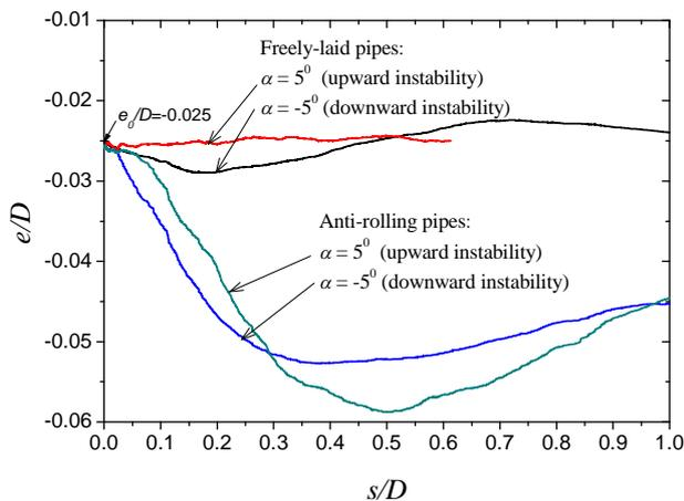
**Fig. 3** Additional embedment vs. lateral displacement while pipe losing stability on a sloping sand-bed ( $D = 0.35$  m,  $W_s = 0.801$  kN/m,  $G = 0.711$ ,  $\mu = 0.32$ ,  $d_{50} = 0.12$  mm,  $D_r = 0.16$ ).
