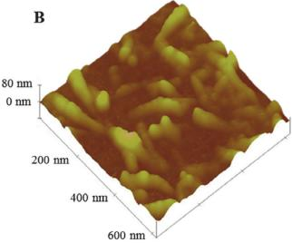
Fig. 3. Morphology images of (A) PAn and (B) PAn-FeTSPP films synthesized under the same conditions as described in Figure 2.
