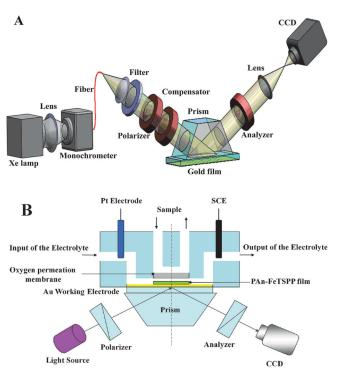
Scheme 2. (A) Scheme of the total internal reflection imaging ellipsometry (TIRIE) system and (B) the electrochemistry-total internal reflection imaging ellipsometry (EC-TIRIE) combination setup.
