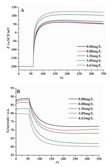
Fig. 6. (A) Electrode potential and (B) grayscale variation with time of the PAn-FeTSPP-modified electrode exposed to different concentrations of DO; Conditions: 0.1 M H<sub>2</sub>SO<sub>4</sub>; initially, E = -200 mV was applied for 60 s followed by the application of a cathodic current of  $I_{appl} = -2.5 \ \mu\text{A}$ .
