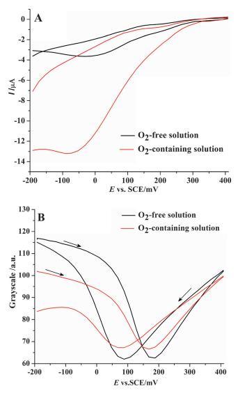
Fig. 4. (A) Steady state polarization curve and (B) simultaneous TIRIE characterization of the PAn-FeTSPP film in 0.1 M  $H_2SO_4$ . The O<sub>2</sub>-containing solution has a DO concentration of ca. 12.8 mg L<sup>-1</sup>.
