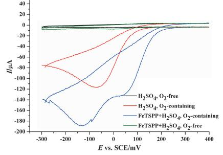
Fig. 1. Cyclic voltammograms of gold film in 0.5 M  $H_2SO_4$  with and without 0.05 mM FeTSPP in  $O_2$ -free and  $O_2$ -containing solution;  $\nu = 20 \text{ mV s}^{-1}$ .
