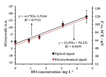
Fig. 7. Electrode potential and grayscale recorded at t=300 s of the PAn-FeTSPP-modified electrode exposed to different concentrations of DO; Conditions: 0.1 M H<sub>2</sub>SO<sub>4</sub>; initially, E=200 mV was applied for 60 s followed by the application of a cathodic current of  $I_{appl}=-2.5 \ \mu$ A.
