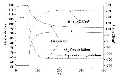
Fig. 5. Real time potential and grayscale curves of PAn-FeTSPP to DO; Conditions: 0.1 M H<sub>2</sub>SO<sub>4</sub>; initially, E = -200 mV was applied for 60 s followed by the application of a cathodic current of  $I_{appl=}-2.5 \mu$ A. The O<sub>2</sub>-containing solution has a DO concentration of ca. 16.5 mgL<sup>-1</sup>.
