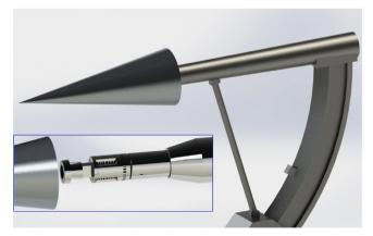
Fig. 1. The model-balance-sting system and its connection detail.
