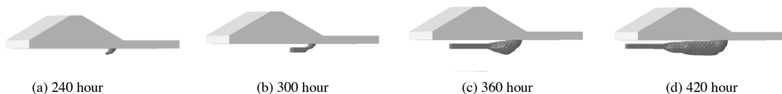
Fig. 4. development of backward erosion pipe
