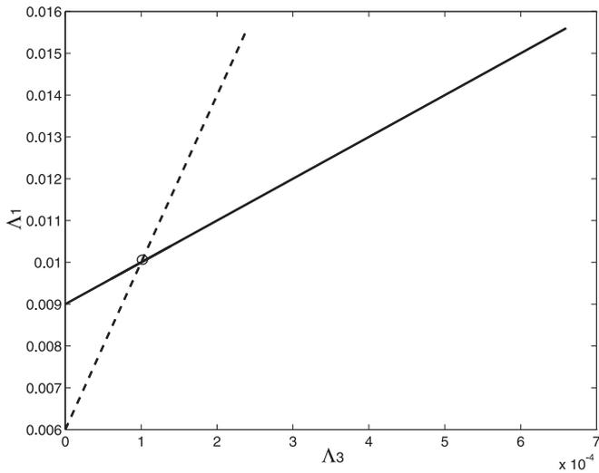
Fig. 4. The projections of the two intersection curves/lines obtained in Figs. 2 and 3 into the  $\Lambda_1 - \Lambda_3$  plane. The intersection of the two curves is marked with a circle, which corresponds to  $(\Lambda_1, \Lambda_3) = (1 \times 10^{-2}, 1 \times 10^{-4})$  exactly.
