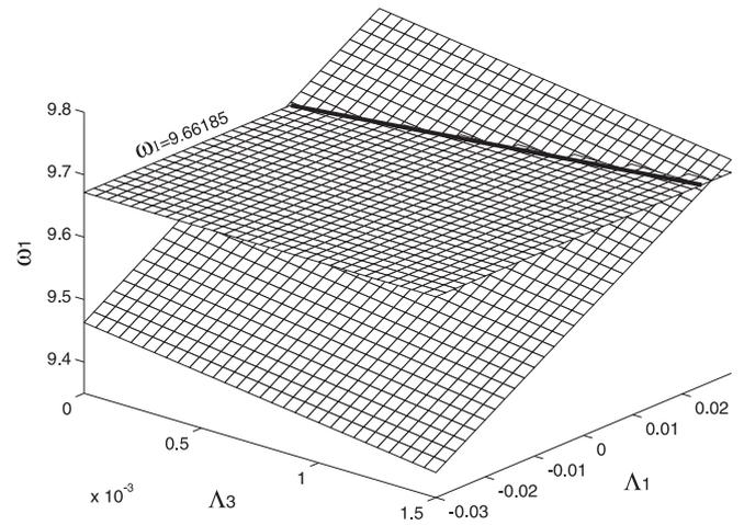
Fig. 2. The variation of the first resonant frequency ( $\omega_1$ ) as a function of  $\Lambda_1$  and  $\Lambda_3$ . The level plane is the one with the constant of  $\omega_1 = 9.66185$ . The intersection of the two planes is marked with a solid line. Here  $\Lambda_2 = -0.5$  is fixed.
