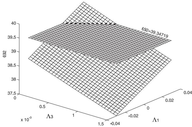
Fig. 3. The variation of the second resonant frequency ( $\omega_2$ ) as a function of  $\Lambda_1$  and  $\Lambda_3$ . The level plane is the one with the constant of  $\omega_2 = 39.34719$ . The intersection of the two planes is marked with a dashed line. Here  $\Lambda_2 = -0.5$  is fixed.
