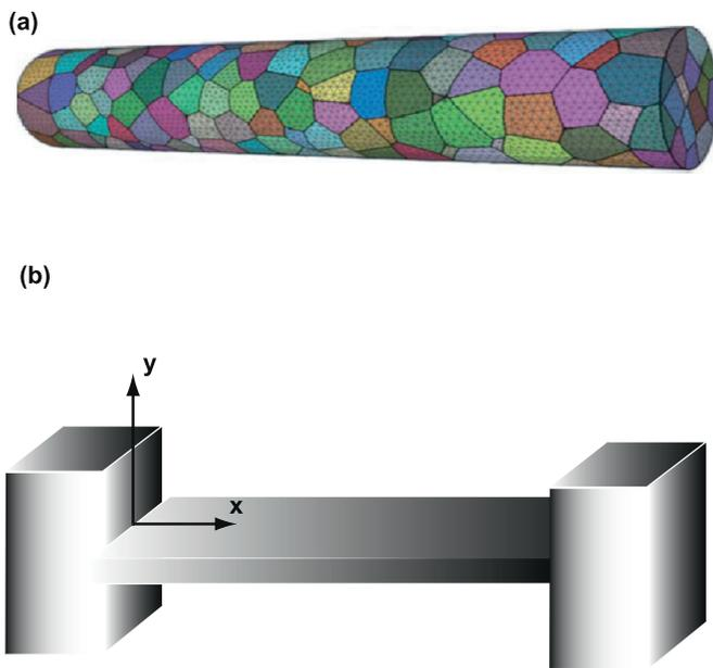
**Fig. 1.** (a) The schematic diagram of a nano-polycrystal beam. Due to the presence of the microstructure of grain and the small size of beam, the properties of inhomogeneity and long-ranged atomic interactions stand out, which leads to the nonlocal effects. (b) The schematic diagram of a clamped-clamped beam and its coordinate system.
