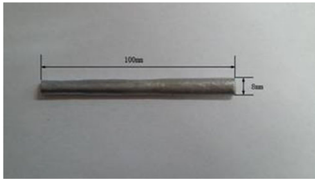
FIG. 3. Typical metal part made by synchronous rolling-casting.
