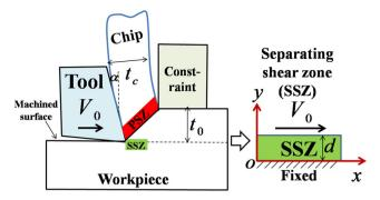
Fig. 7 The schematic of the HSEM model, where the deformation zones of PSZ and SSZ are included
