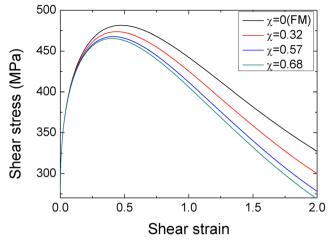
Fig. 8 The calculated stress-strain relations within SSZ for different CEFs  $% \left( {{{\rm{CEFs}}} \right)^{-1}} \right)$
