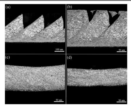
Fig. 3 The microstructures of chips for different CEFs in HSEM AZ31B: a CEF = 0 (FM), b CEF = 0.32, c CEF = 0.57, and d CEF = 0.68
