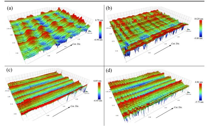
Fig. 5 The digitalized scanned surfaces for different CEFs: a CEF = 0 (FM), b CEF = 0.32, c CEF = 0.57, and d CEF = 0.68
