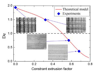
Fig. 9 Comparison of theoretical model with experimental observations for different CEFs
