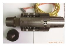
Fig. 5 Six-component stress balance designed for JF12 shock tunnel.
