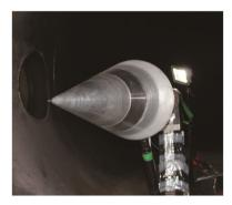
**Fig. 3** 10° half-angle cone model installed in JF12 shock tunnel.
