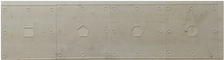
Fig. 6. Experimental specimen of various shape orifices
