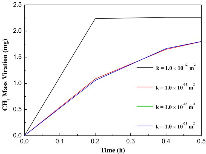
**Fig. 5** CH<sub>4</sub> mass variation versus time for different permeability values
