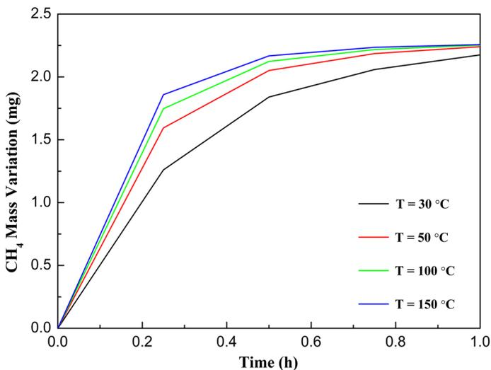
**Fig. 4** CH<sub>4</sub> mass variation versus time for different temperature values
