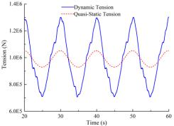
FIGURE 5. TOP TENSION OF THE CATENARY LINE (WITH SPAR SURGE AMPLITUDE=2m, PERIOD=10s)
