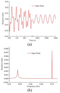
FIGURE 11. THE TIME HISTORY AND FREQUENCY SPECTRUM OF SPAR PITCH (a) THE TIME HISTORY OF PITCH DISPLACEMENT (b) THE FREQUENCY SPECTRUM
