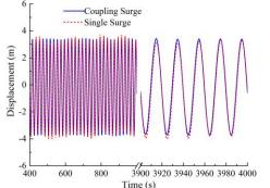
FIGURE 19. THE DYNAMIC RESPONSE OF SPAR SURGE UNDER HARSH WAVE CONDITION
