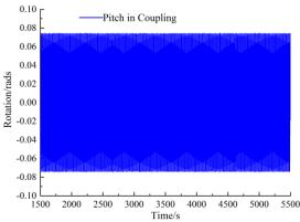
FIGURE 21. LONG PERIOD SPAR PITCH IN COUPLING UNDER HARSH WAVE CONDITION
