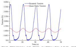
FIGURE 7. TOP TENSION OF THE CATENARY LINE (WITH SPAR SURGE AMPLITUDE=6m, PERIOD=10s)
