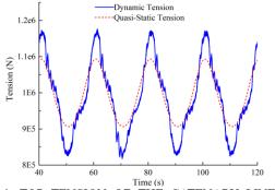
FIGURE 4. TOP TENSION OF THE CATENARY LINE (WITH SPAR SURGE AMPLITUDE=3m, PERIOD=20s)
