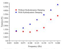
FIGURE 9. EFFECT OF HYDRODYNAMIC DRAG ON MOORING-LINE'S TENSION
