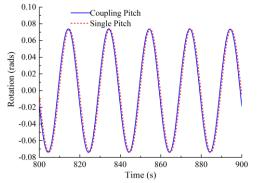
FIGURE 20. THE DYNAMIC RESPONSE OF SPAR PITCH UNDER HARSH WAVE CONDITION
