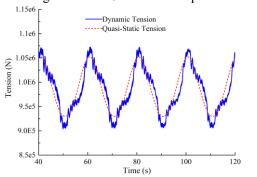
FIGURE 3. TOP TENSION OF THE CATENARY LINE (WITH SPAR SURGE AMPLITUDE=2m, PERIOD=20s)
