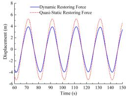
FIGURE 15. THE DYNAMIC RESPONSE, DURING STEADY PHASE, OF SPAR SURGE UNDER WAVE WITH LOWER FREQUENCY
