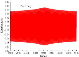
FIGURE 22. LONG PERIOD SPAR SINGLE PITCH UNDER HARSH WAVE CONDITION
