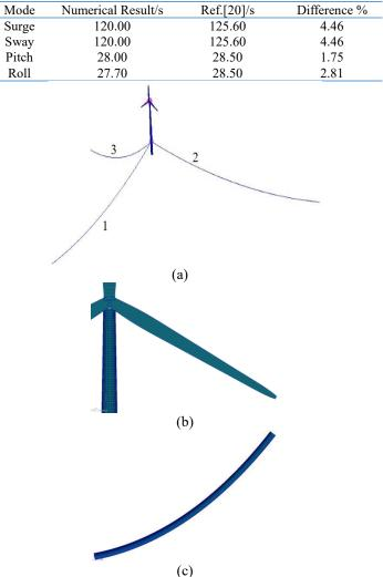
FIGURE 2. THE FEM MODEL OF THE INTEGRATED SYSTEM INCLUDING THE BLADES, TOWER, FLOAGTING SPAR AND CATENARY MOORING-LINES (a) THE INTEGRATED SYSTEM (b) THE PARTIAL ENLARGED VIEW OF BLADES AND TOWER (c) THE PARTIAL ENLARGED VIEW OF A CATENARY MOORING-LINE
