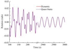
FIGURE 14. THE DYNAMIC RESPONSE OF SPAR PITCH UNDER WAVE WITH HIGHER FREQUENCY
