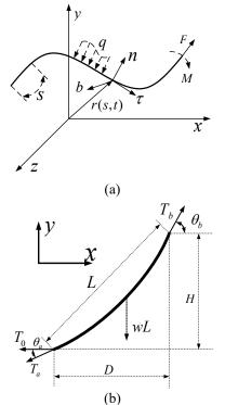
FIGURE 1. CATENARY MOORING LINE (a) THE SCHEMATIC DIAGRAM OF A 3D FLEXIBLE MOORING-LINE (b) THE TRADITIONAL STATIC FORCE BALANCE OF A CATENARY
