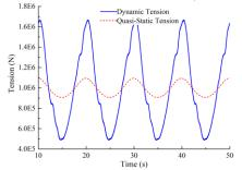
FIGURE 6. TOP TENSION OF THE CATENARY LINE (WITH SPAR SURGE AMPLITUDE=3m, PERIOD=10s)
