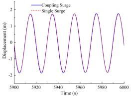
FIGURE 17. THE DYNAMIC RESPONSE OF SPAR SURGE UNDER NORMAL WAVE CONDITION
