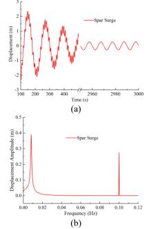
FIGURE 10. THE TIME HISTORY AND FREQUENCY SPECTRUM OF SPAR SURGE (a) THE TIME HISTORY OF SURGE DISPLACEMENT (b) THE FREQUENCY SPECTRUM
