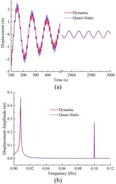
FIGURE 13. THE DYNAMIC RESPONSE OF SPAR SURGE UNDER WAVE WITH HIGHER FREQUENCY (a) THE TIME HISTORY INCLUDING TRANSIENT AND STEADY PHASES, OF SURGE DISPLACEMENT (b) THE FREQUENCY SPECTRUM
