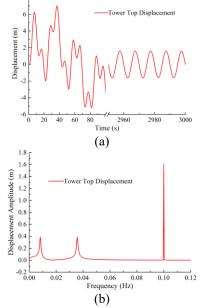
FIGURE 12. THE TIME HISTORY AND FREQUENCY SPECTRUM OF TOWER TOP DISPLACEMENT (a) THE DISPLACEMENT TIME HISTORY (b) THE FREQUENCY SPECTRUM
