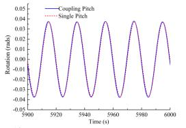
FIGURE 18. THE DYNAMIC RESPONSE OF SPAR PITCH UNDER NORMAL WAVE CONDITION
