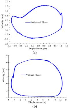
FIGURE 8. PHASE TRACK OF THE VELOCITY VERSUS DISPLACMENT OF THE MIDDLE POINT OF THE CATENARY LINE (a) THE TRACK OF HORIZONTAL MOTION (b) THE TRACK OF VERTICAL MOTION
