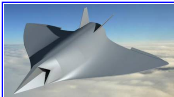
Figure 1. A conceptual configuration of the waverider-based hypersonic vehicles with dorsal mounted engines
