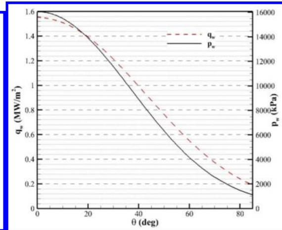
**Figure 8 Sphere wall heat flux and pressure distribution at the condition I, nozzle exit**
