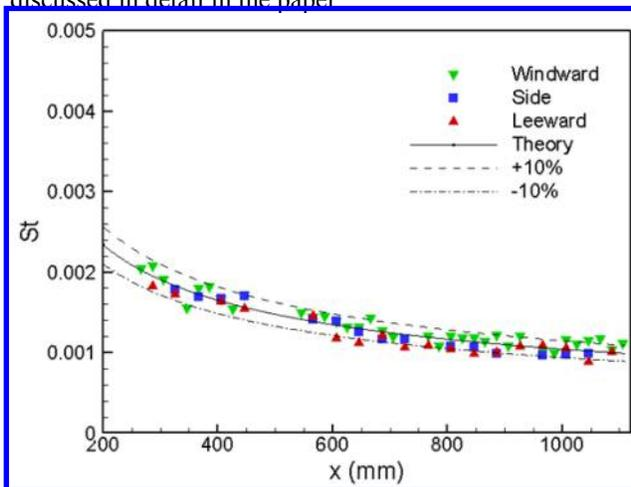
**Figure 9 Heat transfer data comparison between Exp and theory [14]**
