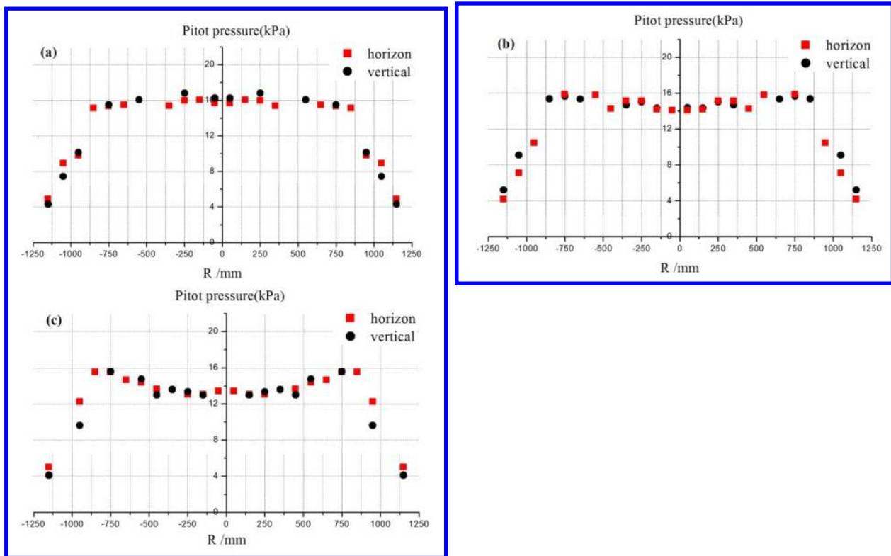
**Figure 6 Pitot pressure distributions for Mach 8 nozzle at the conditions I . (a) cross section 680 mm inside, (b) nozzle exit cross section, (c) cross section 1000 mm outside**
