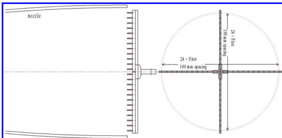
Figure 2 Rake probe configuration used for the flow survey experiments in JF12
