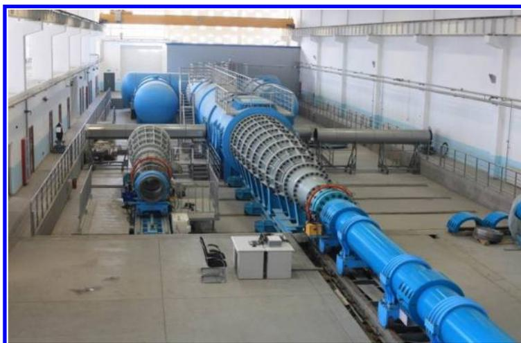
Figure 1 Photograph of JF12 long-test-duration detonation-driven shock tunnel
