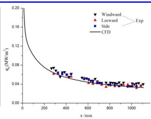
**Figure 10 Heat transfer data comparison between Exp and CFD in JF-12**
