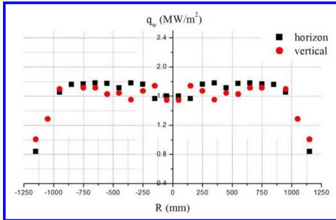
**Figure 7 Heat flux distribution for Mach 8 nozzle at the condition I, nozzle exit**
