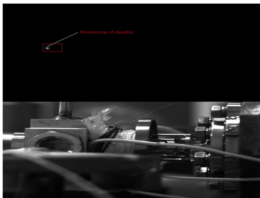
Fig. 8 Radiation image of inner wall: downstream of the thruster chamber.
