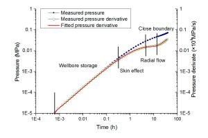
Figure 3. H3-1 pressure drop well-test double logarithmic curves.
