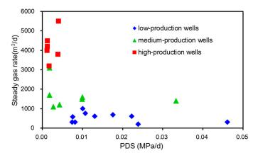
Figure 7. The relation between PDS and steady gas rate in water drainage stage.
