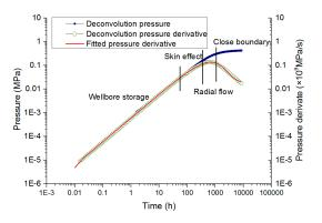
Figure 6. H3-1 deconvolution well-test double logarithmic curve.
