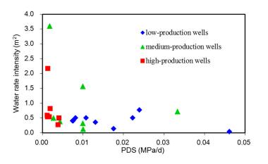
Figure 12. The relation between water rate intensity and PDS in water drainage stage.
