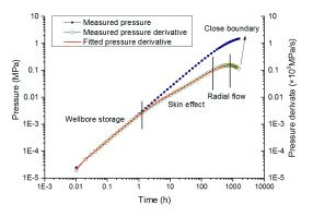
Figure 5. H3-2 pressure build-up double logarithmic curves.
