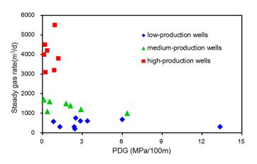
Figure 9. The relation between PDG and steady gas rate in water drainage stage.
