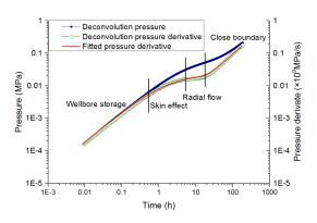
Figure 4. H3-1 deconvolution well-test double logarithmic curves.
