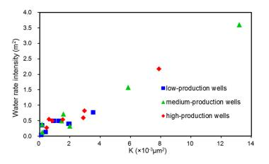
Figure 11. The relation between water rate intensity and permeability in water drainage stage.
