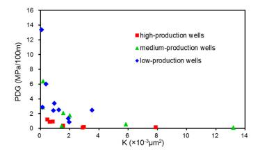
Figure 10. The relation between PDG and permeability in water drainage stage.
