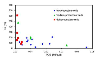
Figure 8. The relation between PDS and investigation radius (Ri) in water drainage stage.
