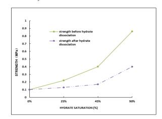
Fig.7 Undrained shear strength of clay containing hydrate before and after hydrate dissociation under  $6_3 = 2.5$ MPa conditions
