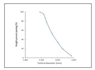
Fig.2 Grain size distribution of clay sediment
