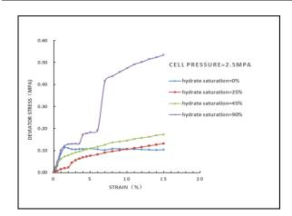
Fig.6 Stress-strain curves of clay sediment samples containing different hydrate saturation after hydrate dissociation under  $\delta_3 = 2.5$ MPa conditions
