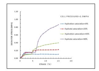
Fig.3 Stress-strain curves of clay sediment samples containing different hydrate saturation under  $\delta_3$  = 2.5MPa conditions
