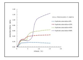
Fig.5 Stress-strain curves of clay sediment samples containing different hydrate saturation under  $\sigma_3 = 7.5$ MPa conditions
