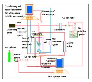
Fig. 1 Sketch of the tri-axial compression test equipment for hydratebearing sediment
