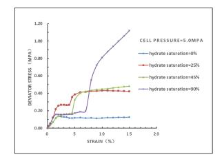
Fig.4 Stress-strain curves of clay sediment samples containing different hydrate saturation under  $\sigma_3 = 5.0$ MPa conditions
