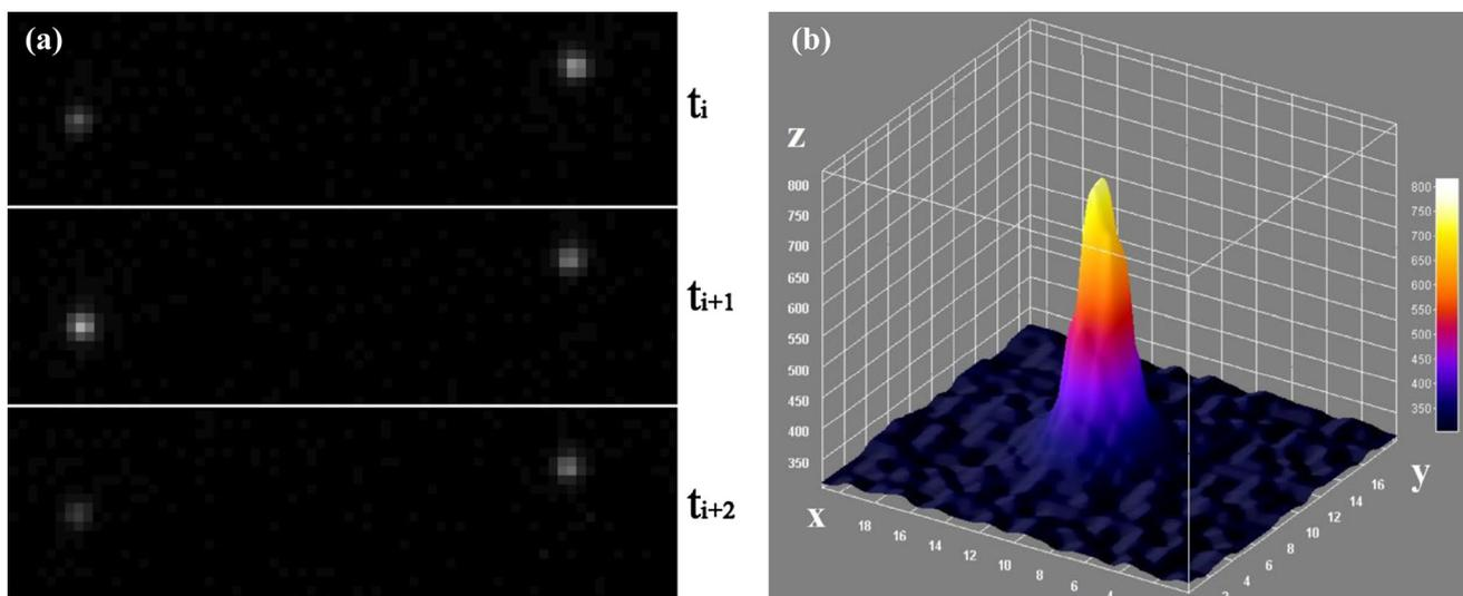
**Fig. 2** **a** Three successive TIRFM images of 100-nm Brownian nanoparticles emerging during the moment  $t_i$  to  $t_{i+2}$  ( $\sim 14$  ms). **b** The intensity distribution of a nanoparticle exhibits a sharp peak, by
