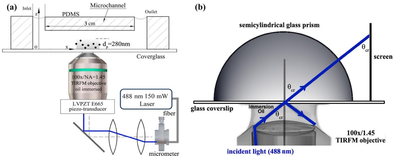
**Fig. 1** Schematic diagrams of **a** the TIRFM experimental system and **b** the calibration of the critical incident angel based on a semi-cylindrical prism
