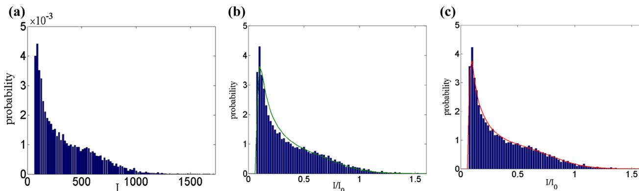
**Fig. 3** The measured histogram and the theoretical prediction of the SID using 100-nm nanoparticles in 1-mM NaCl solution ( $\kappa^{-1} = 10.0$  nm). **a** The measured intensity probability distribution  $p_{\text{exp}}(I)$ . **b** The theoretical result of  $p_{\text{th}}(III_0)$  based on Eq. (5) (the green curve) and the normalized measured data  $p_{\text{exp}}(III_0)$  from **a**. **c** The the-
