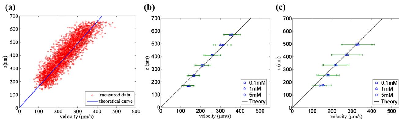
**Fig. 4** Measured velocity profiles using nanoPTV. **a** The scattered velocity data using 250-nm particles in 1-mM NaCl solution. **b** and **c** The measured multi-layer velocity profiles using 250-nm or 100-nm particles, respectively. The blue symbols (rectangles for 0.1 mM, tri-
