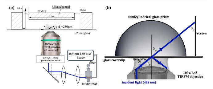
Fig. 1 Schematic diagrams of **a** the TIRFM experimental system and **b** the calibration of the critical incident angel based on a semi-cylindrical prism
