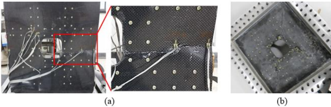
Figure 17 Failure patterns under (a) CLC and (b) SLC
