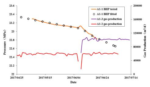
**Figure 4.** A1-1 bottomhole pressure (BHP) fitting results (A1-3 was a new neighboring well produced at June 2017).
