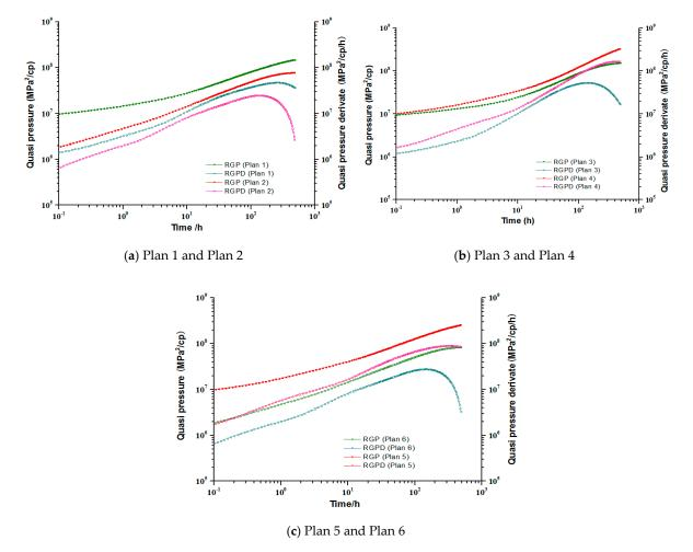
Figure 8. Double logarithmic curve of L2 well recovery pseudo pressure of each plan.
