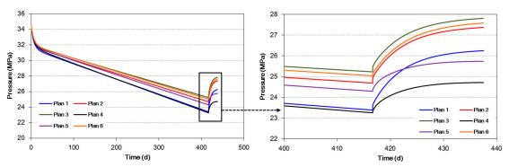
Figure 10. BHP of L2 well after producing 15 months under different well spacing.
