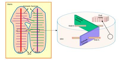
**Figure 1.** Multi-region coupled shale reservoir physical model (Well-A and well-B are two multi-stage fracturing horizontal wells (MFHWs), the hydraulic fractures connected with the SRV and the SRVs are dual medium.).
