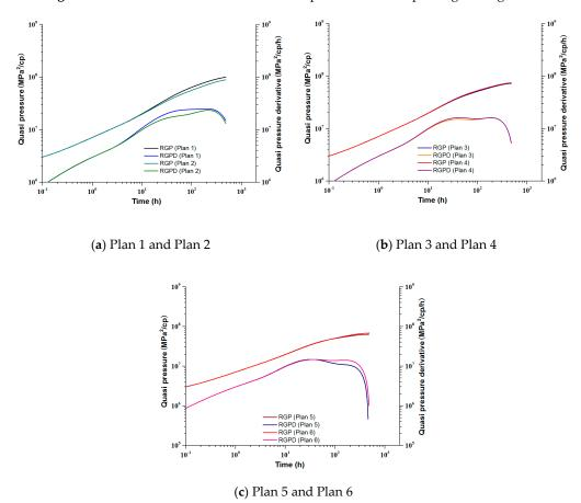
Figure 14. Double logarithmic curve of pressure recovery of shut-in wells under different well pattern and multiple neighboring wells.
