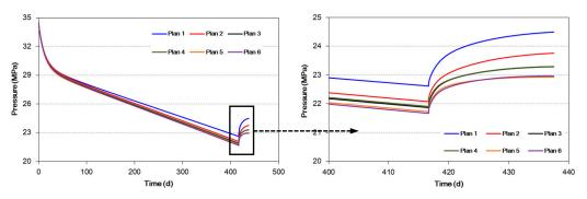
Figure 13. BHP of L2 well with different well pattern and multiple neighboring wells.
