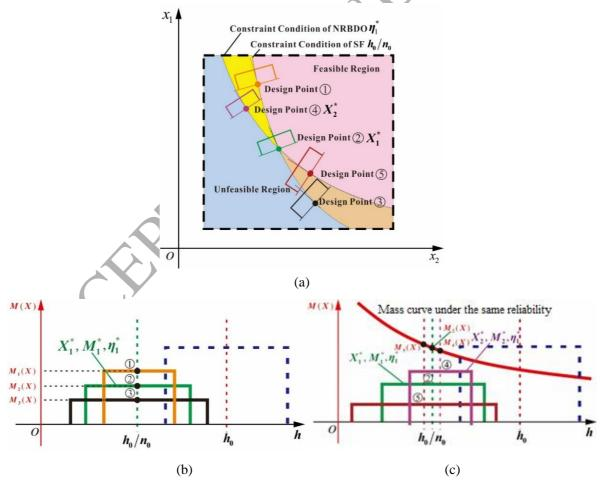
Fig. 5. Comparison of the optimization process between the NRBDO and SF methods: (a) Feasible regions of the two methods, (b) Searching process of the optimal design point of the SF method, (c) Searching process of the optimal design point of the NRBDO method.
