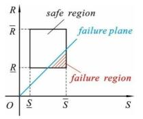
Fig. 1. Nonprobabilistic set-theoretic stress–strength interference model.
