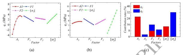
Fig. 15. Sensitivity analysis for the design variables and uncertainties: (a) Effect trends of q<sub>1</sub>; (b) Effect trends of q<sub>2</sub>; (c) Pareto graph for the structural response.
