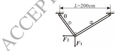
Fig. 8. A two-bar truss structural system.
