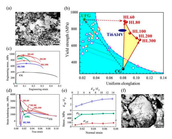
**Figure 2.** Unprecedented strengthening and extra strain-hardening in Ti with heterogeneous lamella structure (HLS): (**a**) Microstructural characteristics of HLS; (**b**) Outstanding tensile properties of Ti with HLS; (**c**) Engineering tensile stress–strain curves for various samples; (**d**) True strain hardening rate vs. true stress for various samples; (**e**) Back stress hardening behaviors for Ti with HLS; (**f**) Dislocation pile-ups at hetero-interfaces. Adapted from [16].
