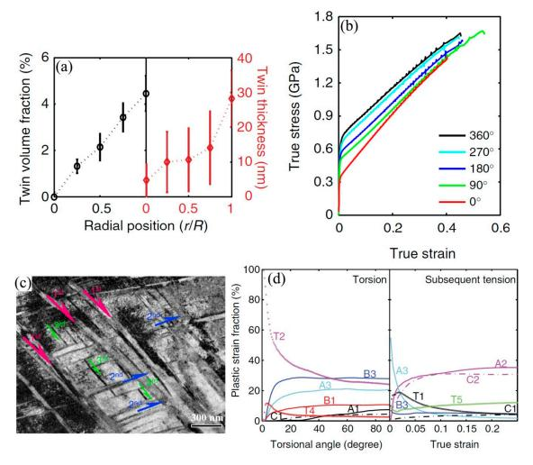
**Figure 7.** Tensile properties and corresponding deformation mechanisms of a TWIP steel with gradient twinned structure: (**a**) Twin volume fraction and twin thickness distributions along the radial direction; (**b**) True stress–strain curves; (**c**) Hierarchical twin structures formed during the pre-torsion deformation and the subsequent tensile loading; (**d**) Activated different twinning systems in the sequential torsion and tension deformation. Adapted from [47].
