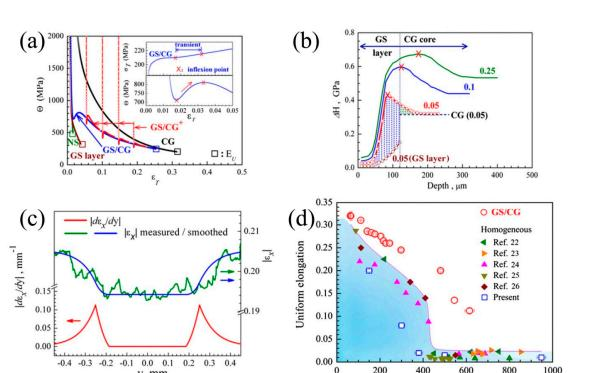
**Figure 6.** Tensile properties and extra strain hardening mechanisms of gradient grained IF steel: (a) Strain hardening rate vs. true strain curves; (b) Extra strain hardening by gradient structures; (c) Distributions of lateral strain and strain gradient along the depth; (d) Superior tensile properties of gradient structures over homogeneous counterparts. Adapted from [14].
