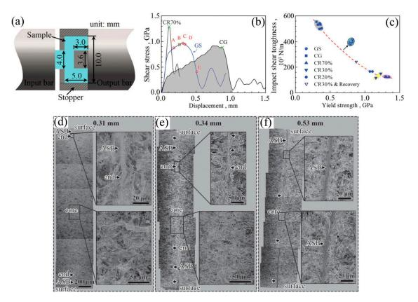
**Figure 9.** Dynamic shear properties and corresponding deformation mechanisms of gradient structure: (a) Set-up of dynamic shear experiments in Hopkinson bar; (b) Shear stress-shear displacement curves; (c) Impact shear toughness vs. dynamic shear yield strength; (d–f) Propagation process of ASB from the surface to the center. Adapted from [58].
