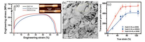
**Figure 5.** Tensile properties and corresponding deformation mechanisms of gradient grained copper: (a) Engineering stress–strain curves; (b) TEM image of the top layer after a true tensile strain of 33% showing "in-situ" coarsened dislocation-free grains; (c) Variation of average grain sizes with applied tensile strain for the gradient layer. Adapted from [42].
