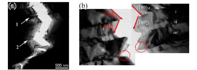
**Figure 14.** In situ TEM images of crack growth process in a thin foil of NT Cu. (**a**) A zigzag crack formed during tensile loading. (**b**) Magnified images of region 1 in (**a**), circles indicate the short crack edges on TBs. Adapted from [107].
