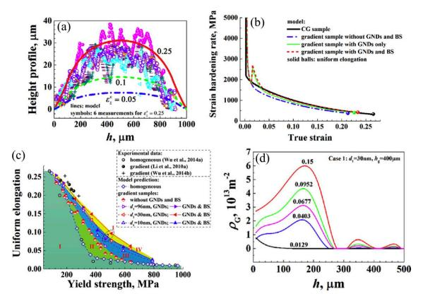
**Figure 11.** Dislocation density-based continuum plasticity modeling for gradient structure: (a) The predicted height profile on the lateral surface of a gradient IF steel and comparison with experimental data; (b) The predicted strain hardening rate and comparison with experimental data; (c) Strength–ductility maps of the gradient IF steel considering GNDs and back stress; (d) The predicted GNDs density distributions for one case. Adapted from [54].
