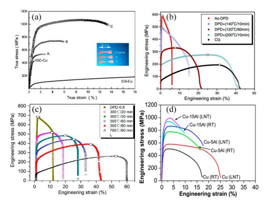
**Figure 12.** Typical tensile strain-stress curves. (**a**) as deposited Cu (adapted from Refs. [75]); (**b**) DPD-Cu (adapted from Refs. [90]); (**c**) DPD-Cu-Zn (adapted from Refs. [80]); (**d**) Cu-Al (adapted from [91]).
