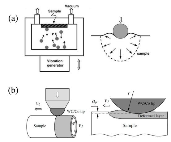
Figure 4. Schematic illustrations of SMAT (a) and SMGT (b) techniques. Adapted from [38] and [41].
