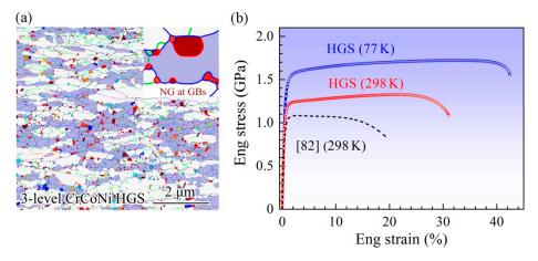
**Figure 1.** Microstructural characteristics and enhanced strength–ductility synergy of the MEA with HGS: (a) Architected HGS; (b) Engineering tensile stress–strain curves for the MEA with HGS under various testing temperatures. Adapted from [17].
