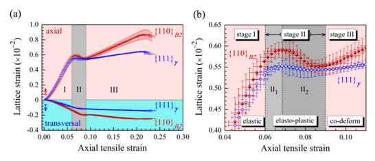
**Figure 3.** In situ x-ray diffraction measurements for the HSSS with HPS during tensile deformation. (a) Lattice strains in both hard B2 phase and soft austenitic matrix vs. applied tensile strain; (b) Close-up view for the transient region. Adapted from [28].
