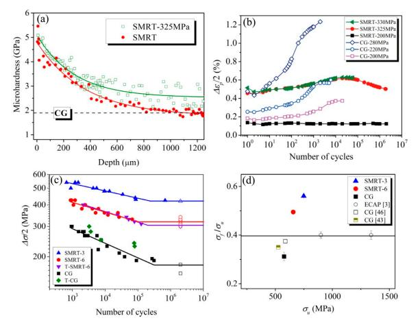
**Figure 10.** Fatigue behaviors of an AISI 316L stainless steel with gradient structure: (**a**) Distributions of microhardness along the depth for different samples; (**b**) Cyclic deformation curves of the CG and the gradient structured samples at different stress amplitudes as indicated; (**c**) S-N curves of different samples; (**d**) Correlation between the tensile strength and fatigue ratio (adapted from [49]).
