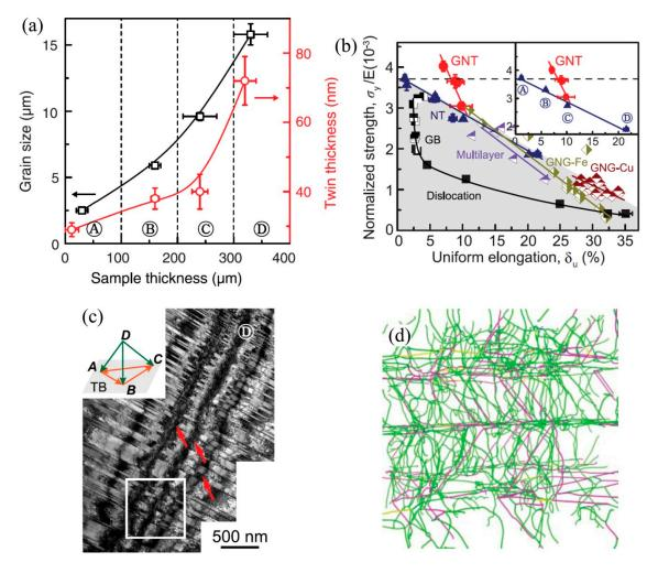
**Figure 8.** Tensile properties and corresponding deformation mechanisms of gradient nanotwinned copper with highly tunable structural gradients: (**a**) Grain size and twin thickness distributions along the thickness; (**b**) Tensile properties; (**c**) Deformation microstructure of gradient nanotwinned structure at 1% strain showing bundles of concentrated dislocations; (**d**) High density of dislocations in the bundles of concentrated dislocations revealed by MD. Adapted from [13].
