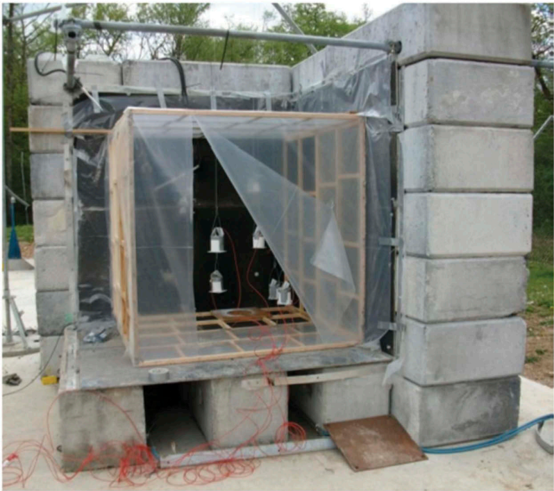
Figure 8. Configuration of the Al/O 2 mixtures detonation experiment.
