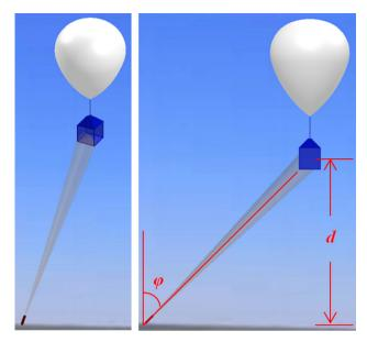
Fig. 1. Sketch of Laser Power Beaming for aerostat.
