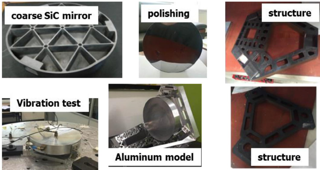
Fig. 5. The development of telescope (up left is the coarse SiC primary mirror, up middle is the polished SiC primary mirror, up right and down right is the SiC telescope structure, down middle is the aluminum telescope model, down left is the vibration test of the aluminum model).
