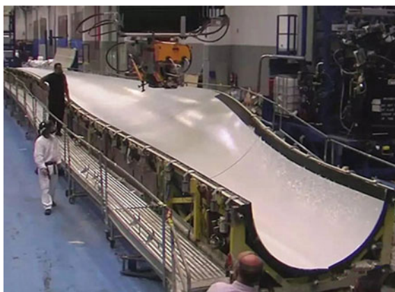
Fig. 6.29 Automatic blade manufacturing system
