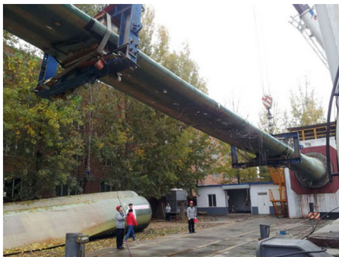
Fig. 6.28 Static test of segmented blades
