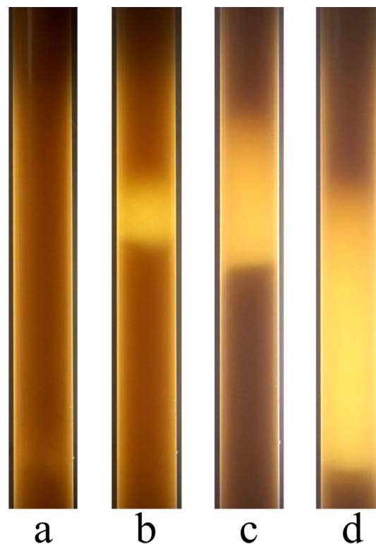
Figure 7. Experimental oil–air two-phase flow behavior observed through a transparent Perspex tube when the superficial gas velocity is 0.17 m/s: (a) bubble flow, u_{sl} = 2.16 m/s, (b) bubble flow, u_{sl} = 1.50 m/s, (c) intermittent flow, u_{sl} = 0.68 m/s, and (d) intermittent flow, u_{sl} = 0.20 m/s.
