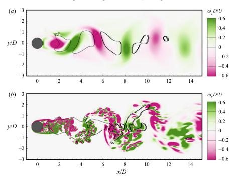
FIGURE 14. Turbulent/non-turbulent interface (solid line) at (a) Re = 100 and (b) Re = 3900identified by SOM. Contours of instantaneous spanwise vorticity  $\omega_z$  are superimposed for comparison.
