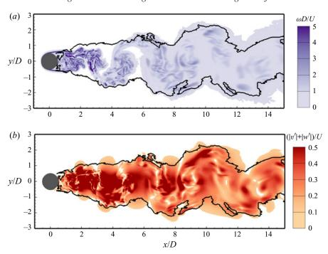
FIGURE 7. Contours of (a) vorticity modulus  $\omega$  and (b) cross-stream fluctuation intensity |v'| + |w'| at Re = 3900. The solid line shows the turbulent/non-turbulent interface identified by the XGBoost detector. Contours for  $\omega < 0.1 U/D$  and |v'| + |w'| < 0.1 U are clipped.
