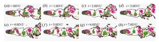
FIGURE 5. Successive snapshots of turbulent/non-turbulent interface (solid line) identified by the XGBoost detector and contours of instantaneous spanwise vorticity  $\omega_z$  at Re = 3900. See figure 4 for the legend of contours.
