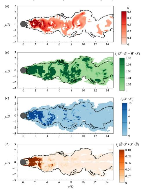
FIGURE 11. Contours of invariants: (a) k, (b)  $I_2(S' \cdot \Omega' + \Omega' \cdot S')$ , (c)  $I_3(S' \cdot S')$  and (d)  $I_2(\bar{\Omega} \cdot S' + S' \cdot \bar{\Omega})$ . Contours corresponding to  $k < 10^{-3}U^2$ ,  $I_2(S' \cdot \Omega' + \Omega' \cdot S')$  $< 10^{-5} U^4/D^4$ ,  $I_3(S' \cdot S') < 10^{-7} U^6/D^6$  and  $I_2(\bar{\Omega} \cdot S' + S' \cdot \bar{\Omega}) < 10^{-5} U^4/D^4$  are clipped. The solid line represents the detected turbulent/non-turbulent interface.
