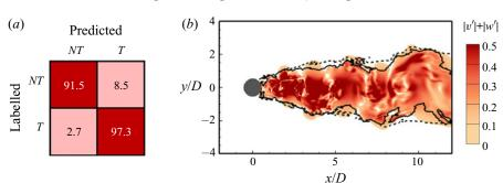
FIGURE 8. Results of detector B. (a) Confusion matrix (see figure 3 for definition); (b) detected turbulent/non-turbulent interface (dashed line). In panel (b), the turbulent/non-turbulent interface identified by detector A as described in §3 (solid line) and the contours of |v'| + |w'| at Re = 3900 are superimposed for comparison.
