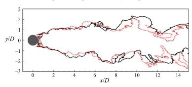
FIGURE 6. Turbulent/non-turbulent interface at Re = 3900 (black solid line) and Re = 5000(red dotted line) identified by the XGBoost detector.
