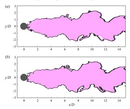
FIGURE 10. Effect of input features on the turbulent region detected by the XGBoost detector. The coloured area shows the detected turbulent region using X (3.1) as the input vector, which consists of eight features, without including the invariants of third-order algebraic polynomials of S' and  $\Omega'$ . The solid line in panels (a) and (b) represents the detected turbulent/non-turbulent interface using  $X^*$  (4.1) and  $X^{**}$  (4.2), respectively, as the input vector.
