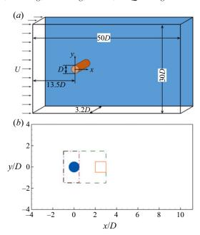
FIGURE 1. Computational domain and coordinate system of DNS and LES of flow past a circular cylinder. (a) Three-dimensional view and (b) two-dimensional view in an x-y plane near the cylinder. The boxes in panel (b) show the regions where training samples are chosen. The samples for the non-turbulent state are chosen from the dashed box for Re = 100 and the dash-dotted box for Re = 3900. The turbulent samples are chosen from the solid box for Re = 3900.
