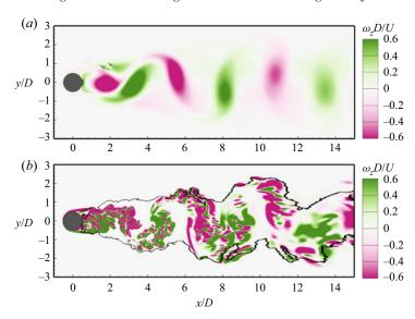
FIGURE 4. Turbulent/non-turbulent interface (solid line) at (a) Re = 100 and (b) Re = 3900identified by the XGBoost detector. Contours of instantaneous spanwise vorticity  $\omega_z$  are superimposed for comparison.
