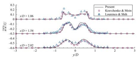
FIGURE 2. Transverse profiles of the mean square of streamwise velocity fluctuations u'u' at three downstream locations in the wake of a circular cylinder at Re = 3900.
