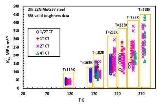
Fig. 7—All 555 valid data points of cleavage fracture toughness (Data listed in Ref. 16).
