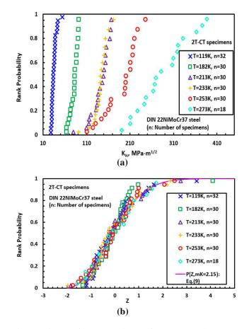
Fig. 11—Cleavage fracture toughness of 2 T CT specimens: (a) experimental data (Data listed in Ref. [16]), (b) standardized distribution of cleavage fracture toughness.
