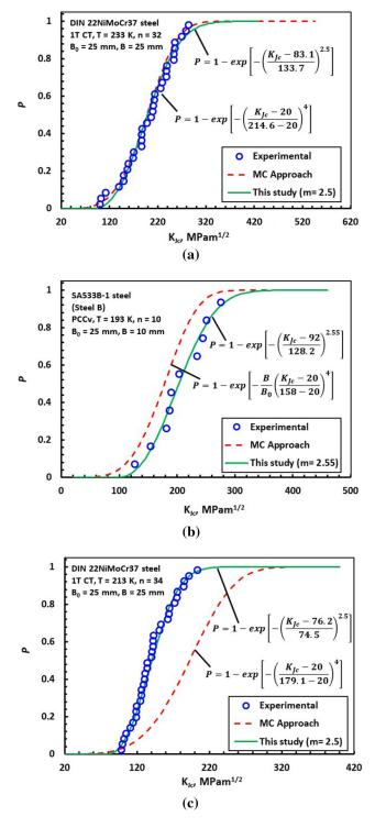
Fig. 17—Typical scenarios of data fitting by the Master Curve (MC) approach and comparision with the proposed approach: (*a*) close esimate by MC, (*b*) overestimate by MC; (*c*) underestimate by MC, (*d*) inconsistent estimate by MC.
