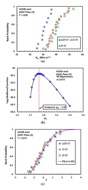
Fig. 4—(*a*) Experimental data of cleavage fracture toughness  $K_{\rm JC}$  of A533B Cl.1 steel measured with 0.5 T, 1 T and 2 T specimens at 123 K (data listed in Ref. 14], (*b*) maximum likelihood estimate of Weibull modulus  $m_K$  using all 38 experimental data, (*c*) comparison of experimental  $K_{\rm JC}$  distribution with estimation.
