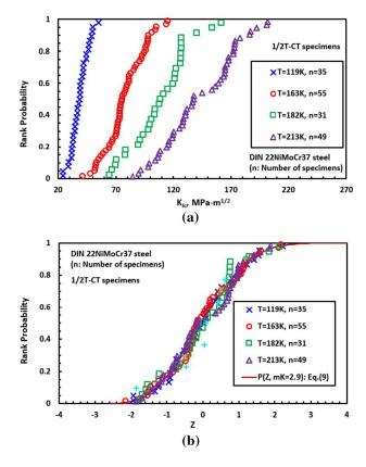
Fig. 9—Cleavage fracture toughness of 1/2 T CT specimens: (a) experimental data (Data listed in Ref. [16]), (b) standardized distribution of cleavage fracture toughness.
