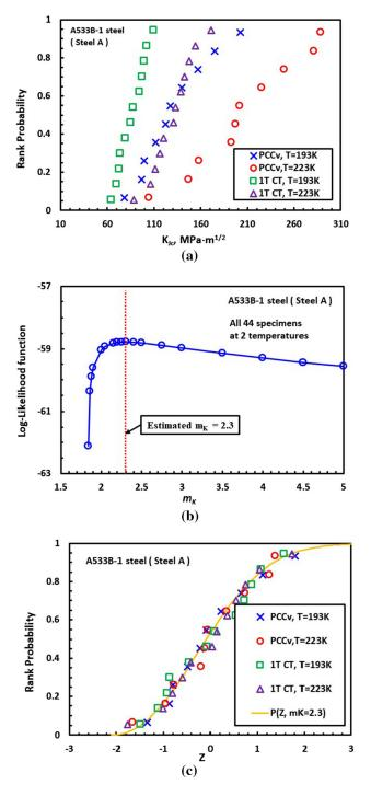
Fig. 5—(*a*) Experimental data of cleavage fracture toughness  $K_{JC}$  of A533B-1 steel (Steel A) at different temperatures (data listed in Ref. 15), (*b*) maximum likelihood estimate of Weibull modulus  $m_K$  using all 44 experimental data, (*c*) comparison of experimental  $K_{JC}$  distribution with estimation.
