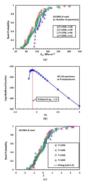
Fig. 3—(*a*) Experimental data of cleavage fracture toughness  $K_{JC}$  of SA738Gr.B steel measured with 1T-CT specimens at different temperatures (data listed in Ref. [13]), (*b*) maximum likelihood estimate of Weibull modulus  $m_K$  using all 116 experimental data, (*c*) comparison of experimental  $K_{JC}$  distribution with estimation.
