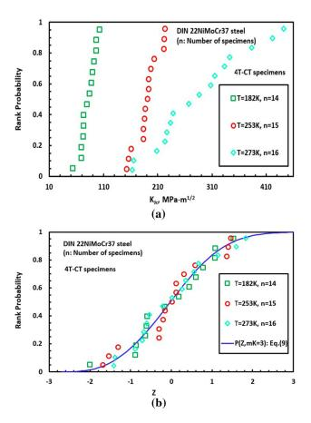
Fig. 12—Cleavage fracture toughness of 4 T CT specimens: (a) experimental data (Data listed in Ref. [16]), (b) standardized distribution of cleavage fracture toughness.
