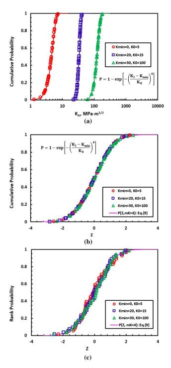
Fig. 2—Three cleavage fracture toughness distributions all with  $m_K = 4$  but different  $K_0$  and  $K_{min}$ : (a) Raw toughness data, (b) the standardized formats with population mean and standard deviation, (c) the standardized formats with sample average and standard deviation, (d)  $\hat{m}_K$  vs number of data sets, (e) maximum likelihood estimation with all three data sets as input.
