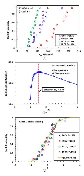
Fig. 6—(*a*) Experimental data of cleavage fracture toughness  $K_{JC}$  of A533B-1 steel (Steel B) at different temperatures (data listed in Ref. 15], (*b*) maximum likelihood estimate of Weibull modulus  $m_K$  using all 44 experimental data, (*c*) comparison of experimental  $K_{JC}$  distribution with estimation.
