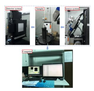
of 23 Lp/mm. The exact resolution of the backfill specimen prepared in the experiment was 68  $\mu$ m. Figure 5 presents a diagram of the CT test system device.
