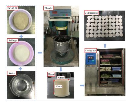
Figure 3. Preparation process of CTB specimens.
