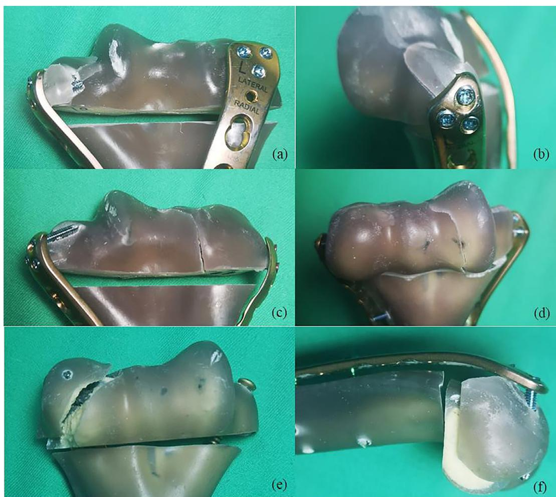
**Fig. 7.** Examples of construct failure when screw cutting-out and fractures occur. Three types are included: (a) (b) “distal medial failure”; (c) (d) “distal medial and trochlear failure”; (e) (f) “capitellar failure”.
