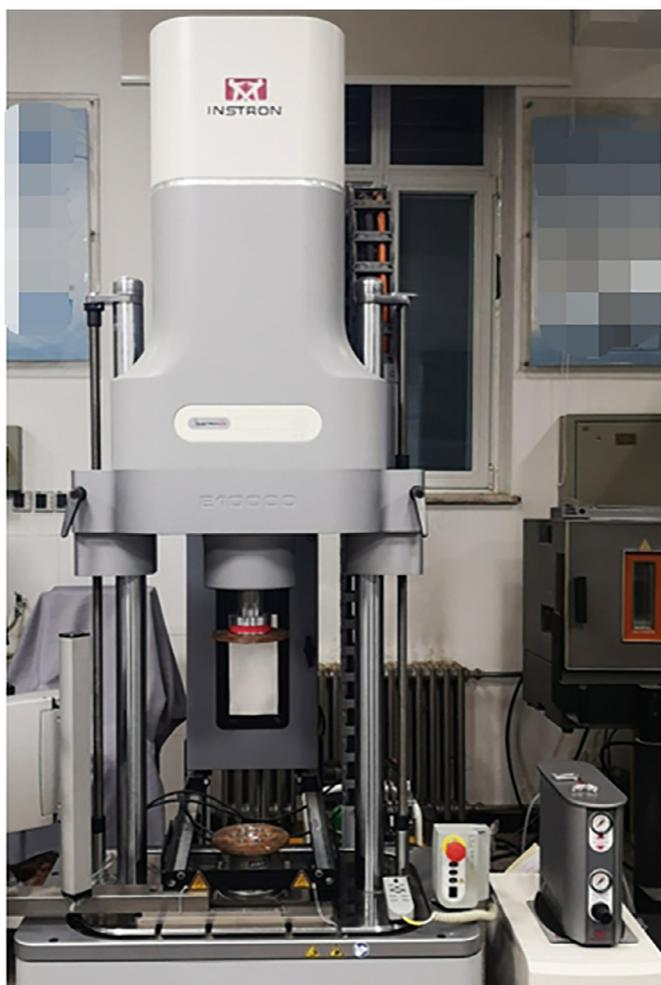
Fig. 3. Universal material testing machine (INSTRON ElectroPuls™ E10000, Norwood, MA, USA).
